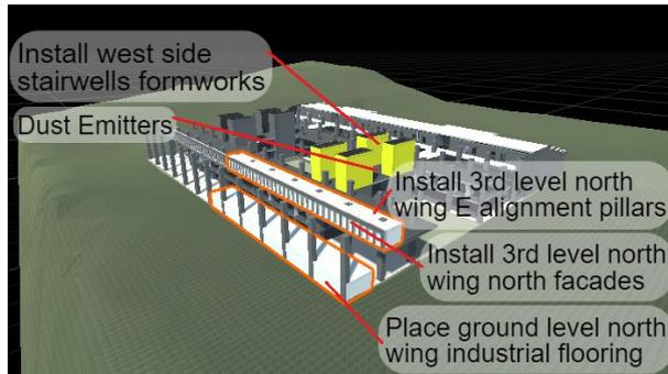
Figure 3. Construction site use case with workspaces and dust emitters.
